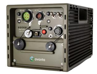
The avanta UPS is a configurable, modular, EMI silent power supply. With dual 90 to 264V AC and wide range 18 to 38V DC inputs, the UPS will provide a 28V output from all sources.
