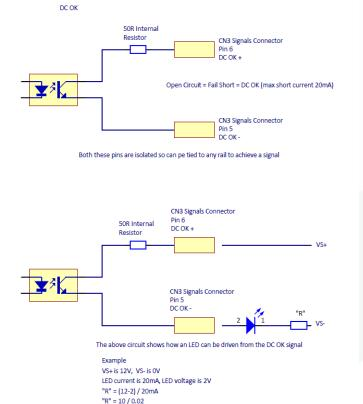
Placing a 500 ohm resistor in series with a 20mA LED will provide a DC OK
